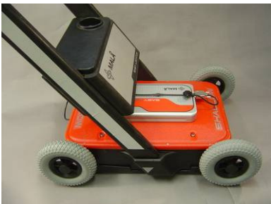
Fig.2.4 Left: Shaft mounted to the antenna. Right: Securing pins.
