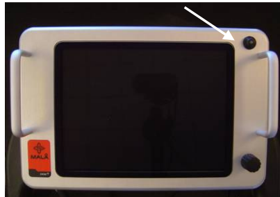
Fig 2.8. Start button on the control unit (left) and the monitor (right)
