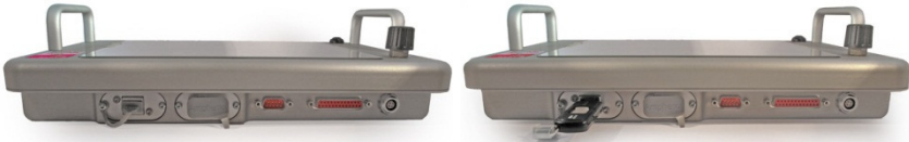
Fig. 3.1. Left: Rubber lid covering the USB port. Right: Connected USB-memory stick.
