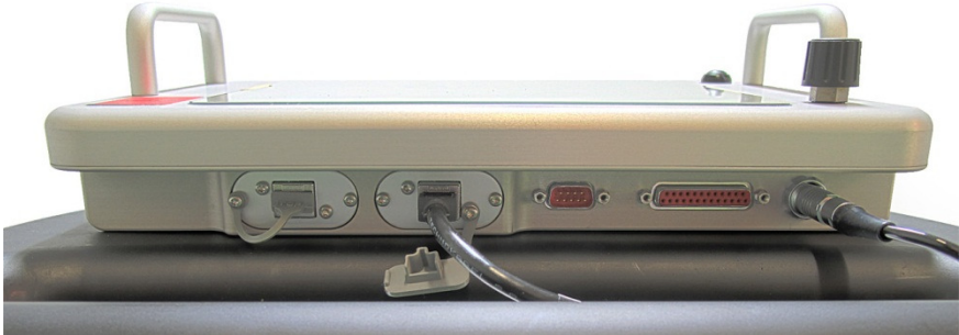
Fig. 2.5 Connections on the monitor; to the left, the Ethernet cable and to the right, the power cable.
