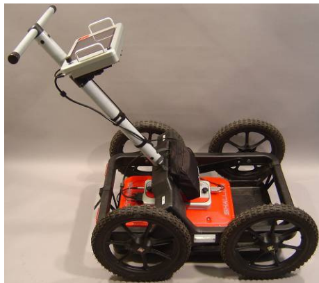
Fig.2.5. The Easy Locator antenna, control unit and monitor on a RTC.
