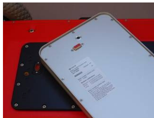
Fig. 2.10. Under side of the control unit showing one of the two connectors that should be fitted on the antenna unit.
