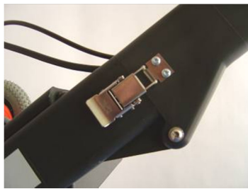
Fig.2.3 The foldable shafts unlocked (left) and locked (right).
