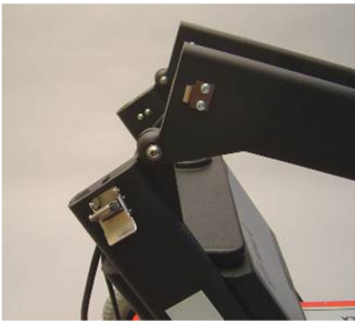
Fig.2.3 The foldable shafts unlocked (left) and locked (right).
