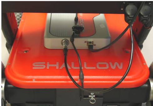
Fig. 2.6. The connections to the control unit; left is power and right is Ethernet communication cable. Above right the connections to the battery box is seen.
